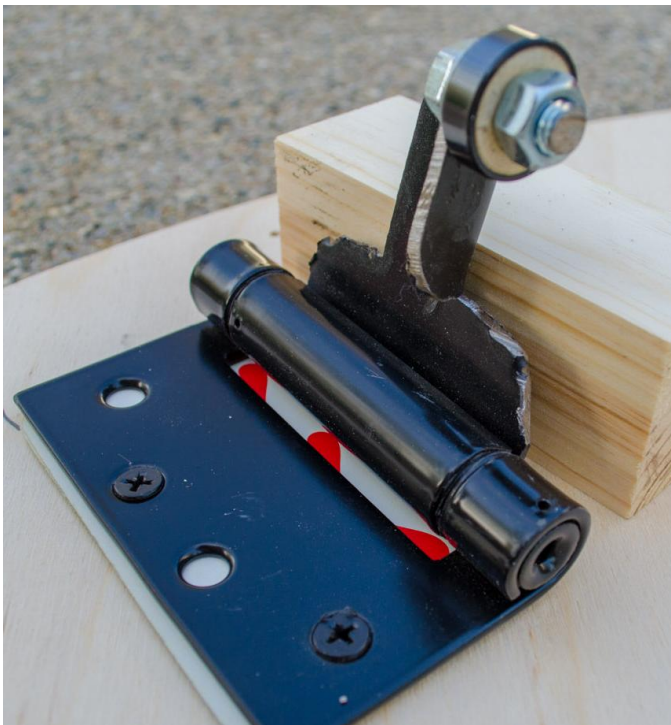
Figure 70: Roller Open Detail
