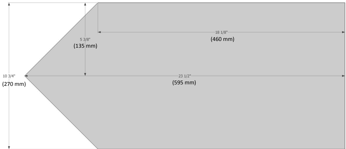
Figure 42: Raising Surface Top View
