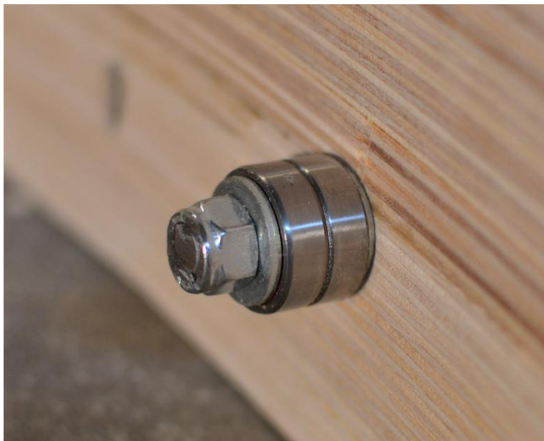
Figure 68: Skirt Roller/Bearing Closeup
